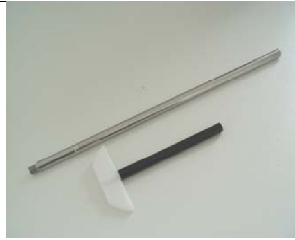
st.st. Stirring Shaft # 316-0116-6 Ctd. Paddle Adapter # 316-0250-6
